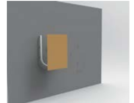
9. Removal of the cardboard support.
