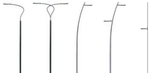
pole with single arm pole with double arm tapered curved pole tapered curved pole with intermediate fitting wall attachment
